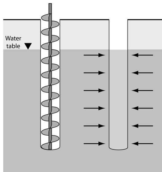
Figure 4. Auger-hole method for water sampling. Sample is bailed from open auger hole.
