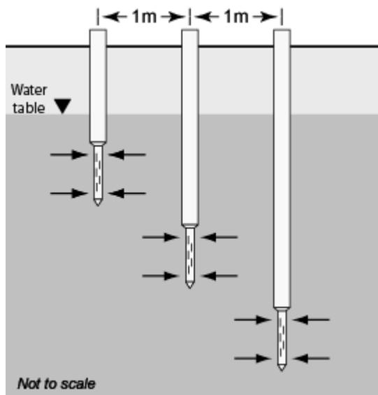
Figure 3. Profile sampling using direct-push tooling. Sample is bailed from slotted inner rod.
