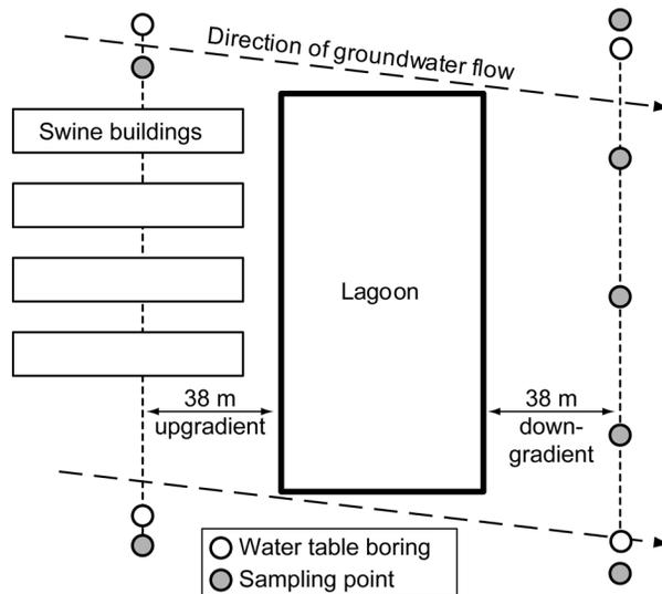
Figure 1. Layout of sampling points on a typical lagoon site.
