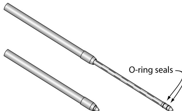
Figure 2. Direct-push tooling used for groundwater sampling. Top: slotted inner rod extended for water collection. Bottom: slotted inner rod retracted for driving to sampling depth.
