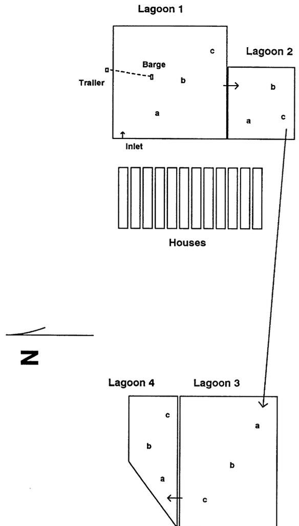
Fig. 1. Schematic diagram of swine production facility. Lagoons 1 and 3 are 3.5 ha and lagoons 2 and 4 are 1.3 ha. Approximate location of temperature sensors and gas collection carboys are indicated by the letters a, b, and c in each lagoon.
