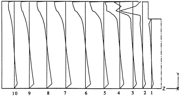
**Figure 2 Velocity profile at the middle of the cross section of pen No. 10**
