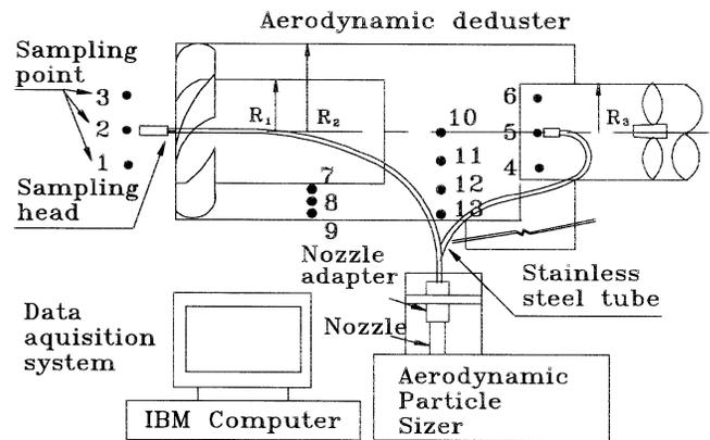
The drop in air velocity and pressure were measured using a hot wire anemometer. Air velocity was measured at all points shown in Figure 4 (numbered 1 to 13). Total pressure drop across the deduster was measured at points numbered 4, 5 and 6.
