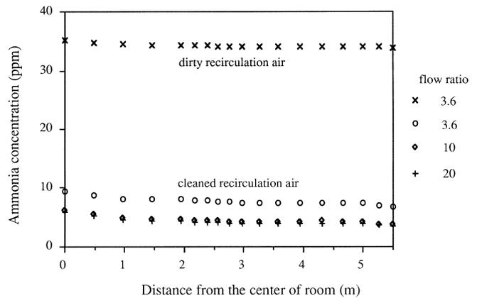
**Figure 7. Effect of the placement of inlet slots on the ammonia contaminate distribution along the human breathing line.**
