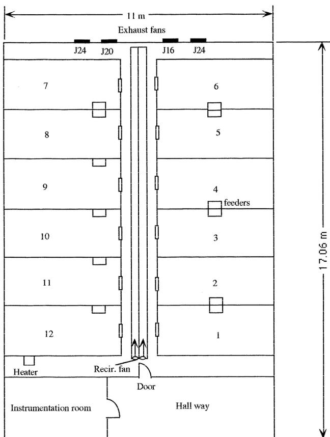
**Figure 1** The floor plan of the grower-finisher room and adjacent areas
