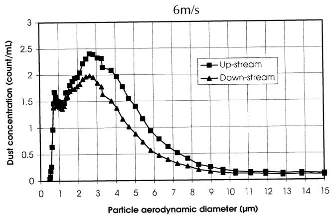
Figure 6 shows the calculated results of dust separation efficiency. Dust separation efficiency increased for particles ranging from 1.5  $\mu\text{m}$  to 6  $\mu\text{m}$  at the three air flow speeds measured. For example, separation efficiency was 10% to 20% for particles of 2  $\mu\text{m}$  and 30% to 37% for particles of 5  $\mu\text{m}$  diameter. Dust separation efficiency appeared unstable for particles larger than 6 and 10  $\mu\text{m}$
