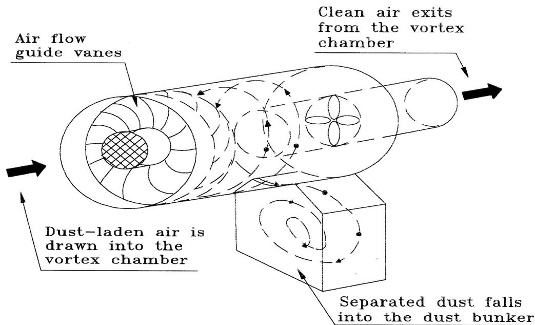
**Figure 1. A sketch of the uniflow aerodynamic deduster prototype**
