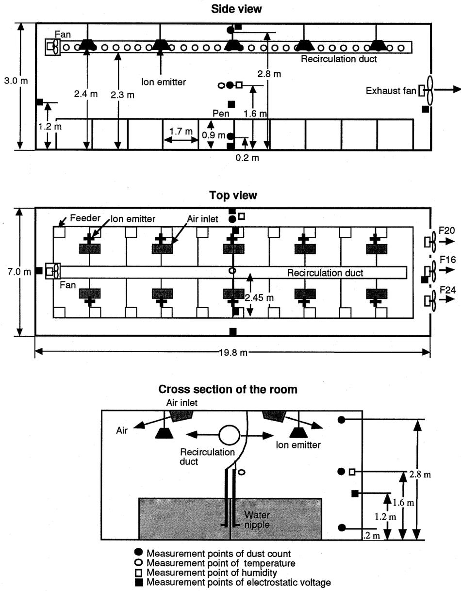
Figure 1. Sketch of the experimental room and measurement points.
