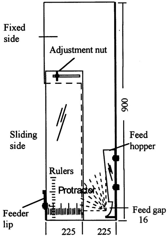
Figure 1. Experimental feeder (measurements in mm)
