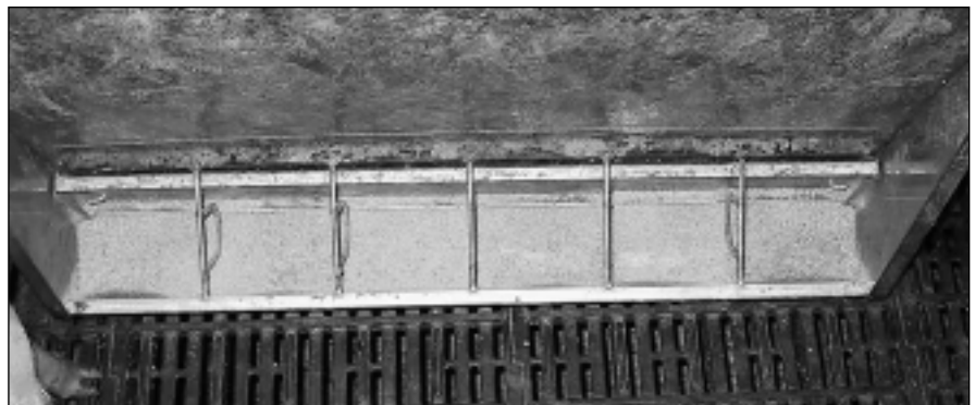
Figure 3 Feeder trough coverage with a gap adjustment providing a gap opening of 31.5 mm.
