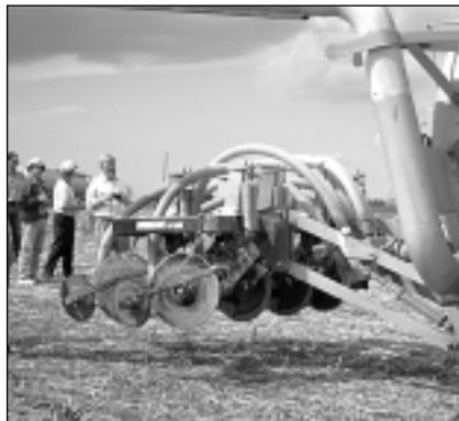
Figure 1 Low disturbance coulters system for injecting liquid manure into forage stands and no-till fields.
