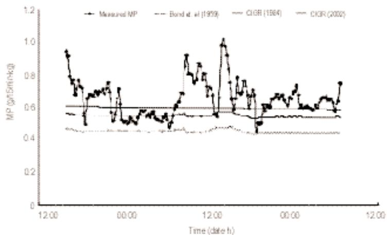
Figure 2: Measured moisture production (MP) and calculated MP for grower pigs (43-45 kg) on dry feeders in the second experiment in g/15 min/kg.
