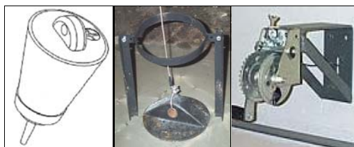
Figure 1. Improved pit-plug design showing the (a) extended cone plug, (b) with cable attached and plug-height stop, and (c) the cable-winch system for remotely pulling the plug from outside the room.
