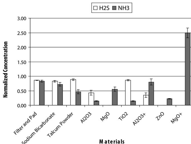
**Figure 1.** Average normalized concentrations of target gases passed through various powder materials. Each value is the average of three replicates and the error bars represent standard error of the mean.
