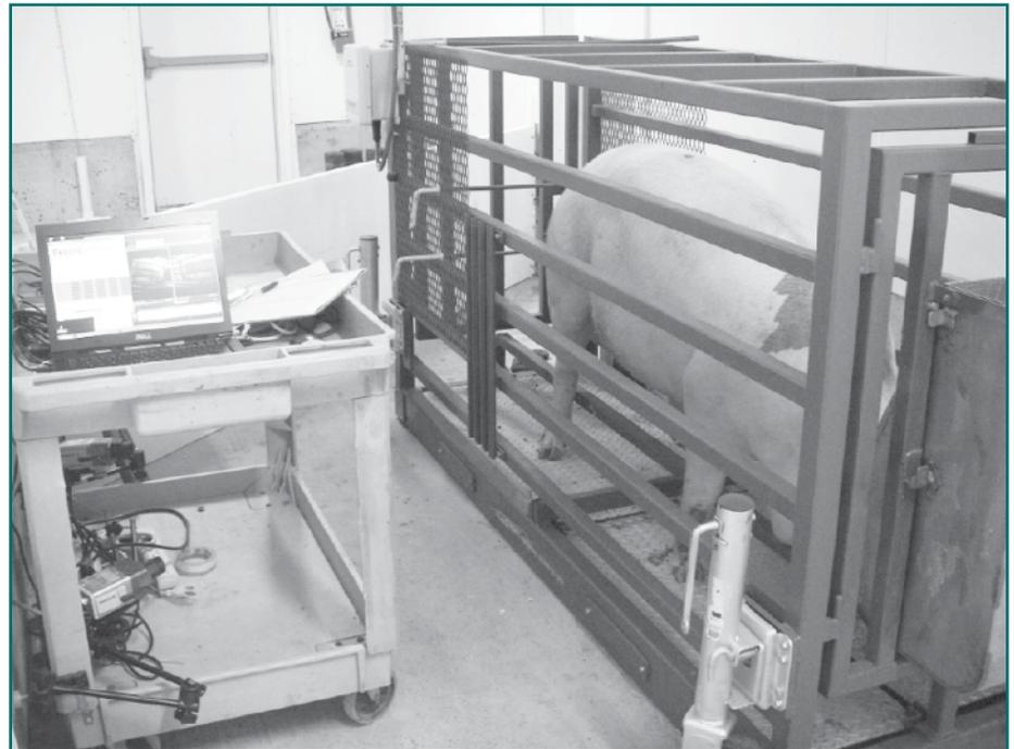
**Figure 1. Sow standing in the force plate**
