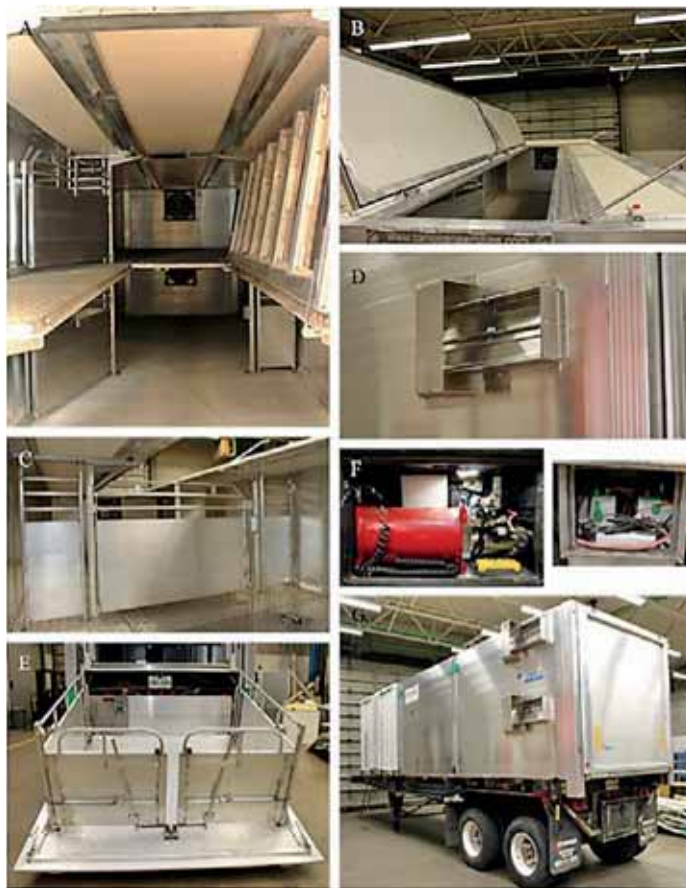
Figure 1. Photos of the animal compartment showing (A) its lower and upper decks, (B) hinged roof, (C) gate that partitions each deck into two compartments, (D) air exhaust damper, (E) hydraulic loading platform, (F) hydraulic system showing motor, pump, controller and power supply, and (G) exterior of the assembled compartment.
