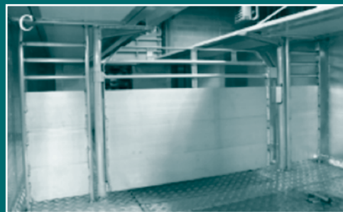
(C) gate that partitions each deck into two compartments
