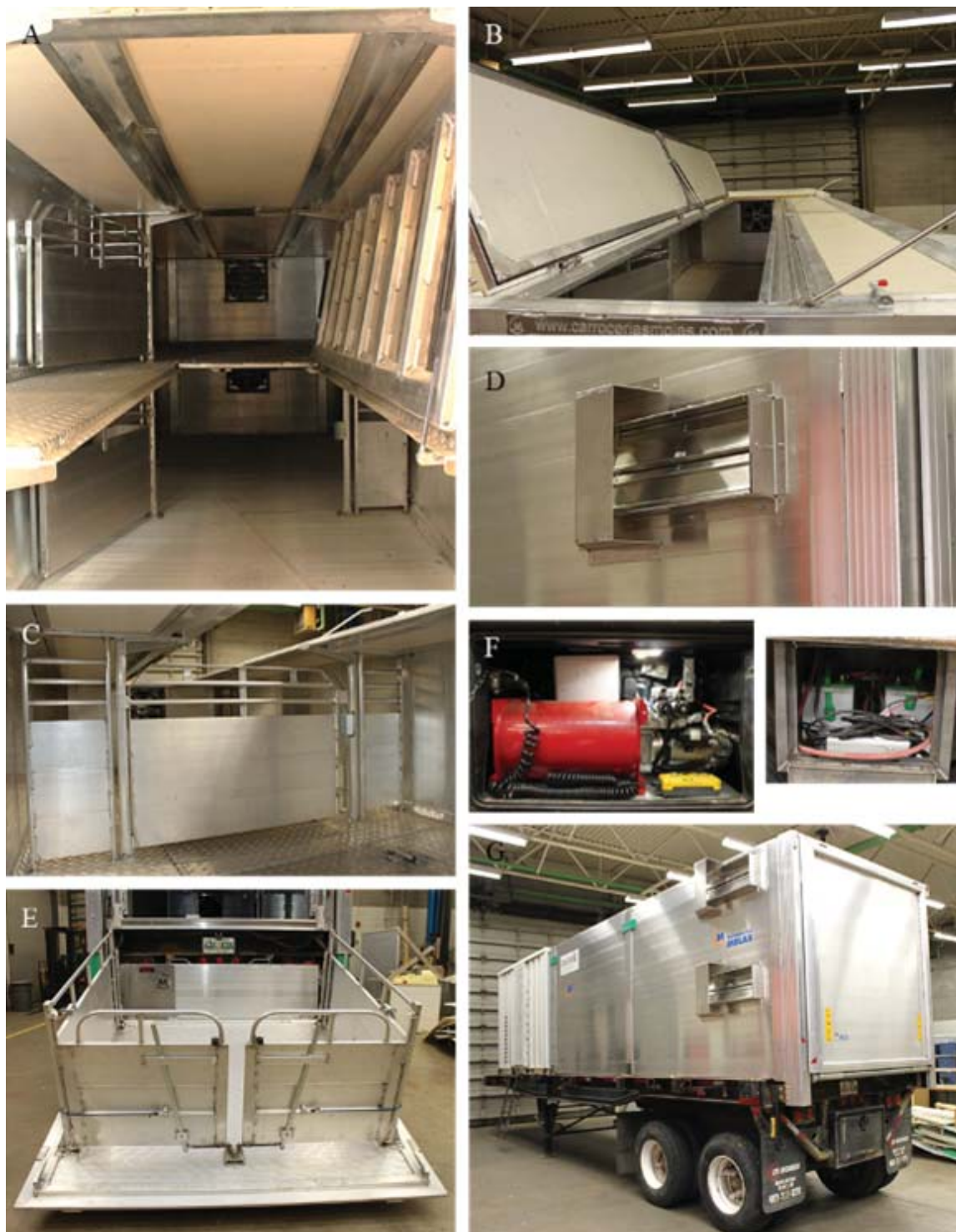
Figure 2. Photos of the animal compartment showing (A) its lower and upper decks, (B) hinged roof, (C) gate that partitions each deck into two compartments, (D) air exhaust damper, (E) hydraulic loading platform, (F) hydraulic system showing motor, pump, controller and power supply, and (G) exterior of the assembled compartment.
