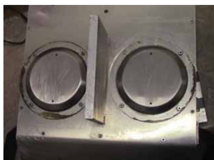
Figure 1. The operant panel containing two identical buttons, a central divider, and a light to indicate when the panel is active.
