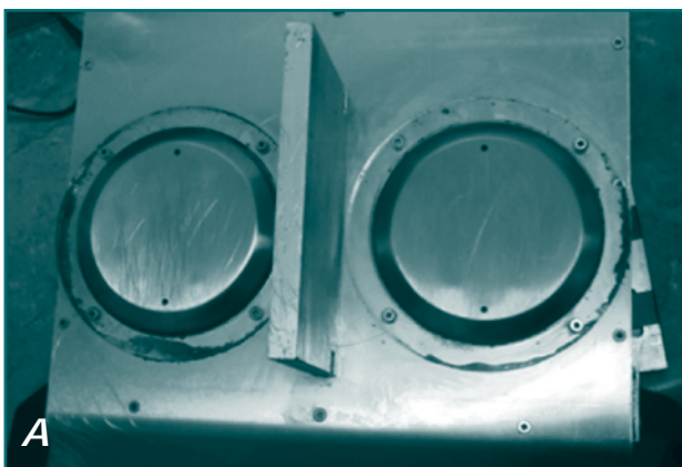
Figure 1. A) The operant panel containing two identical buttons, a central divider, and a light (central dot above divider) to indicate to the sow when the panel is active. B) Sow pressing the active button (results in a reward) of the operant panel, hung over her stall gate.
