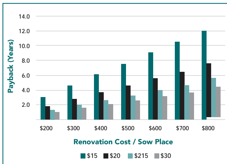
Figure 6. Impact of Labour Rate ($/hour) and Renovation Cost ($/sow place) on payback (time) required in making the conversion to group sow housing.
