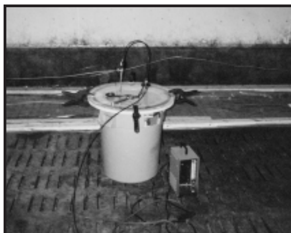
Sampling setup for odour and gas measurements. The apparatus sits on top of the slats, with sampling tubes going down to just above manure level.
