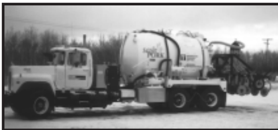
PAMI's tanker truck injector system is based on a Mack tractor unit with a stretched frame.
