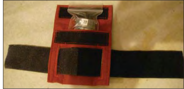
Figure 3. Hobo accelerometer inside a pouch to be held around the lower hind leg
