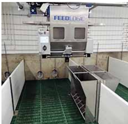
Feed Logic system. The automated feed delivery robotic system keeps track of feed delivered to each pen accurately. The robotic system manages multiple diets and can also blend feeds or dispense supplements or additives to specific pens with no cross contamination.
