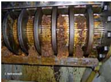
Figure 1. Expeller-pressing canola seed. The seed is pressed by a rotating screw with narrowing flight against a barrel made of steel bars. Oil drips at the bottom; cake comes out at the other end. Photo by E. Beltranena®.
