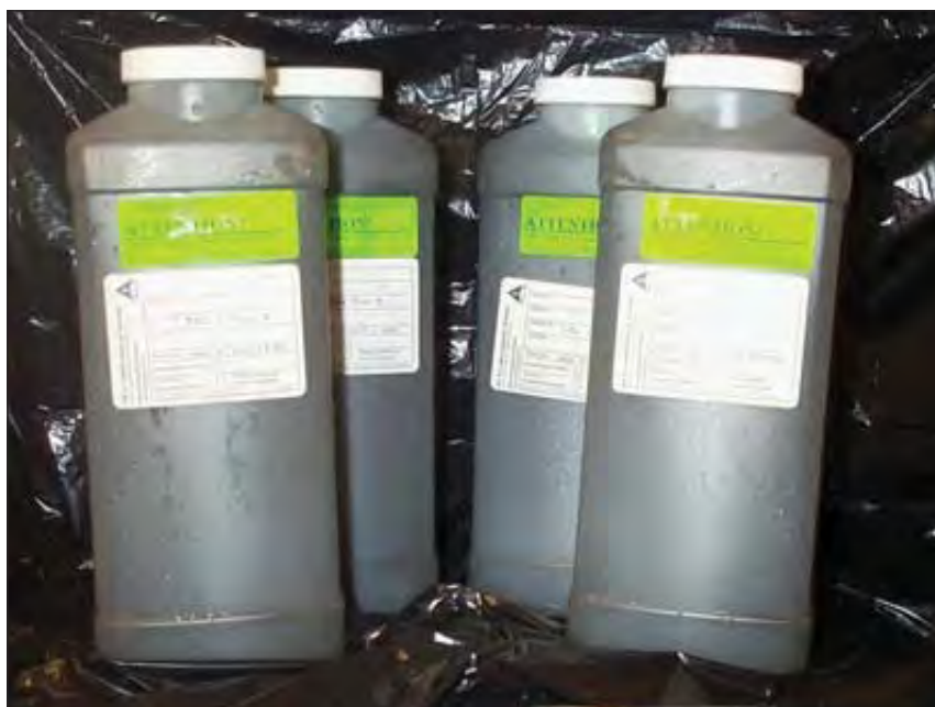
Manure samples collected from the manure tub of each chamber during room-scale tests. These samples were sent to a commercial laboratory for analysis.
