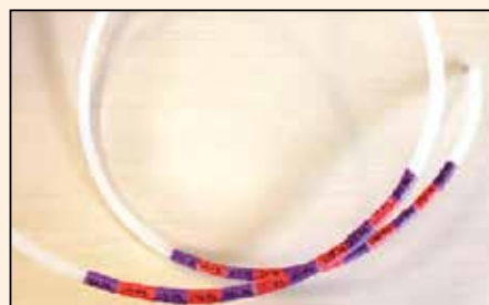
Figure 2: Polyethylene tube designed to estimate body weight using heart girth measurements.
