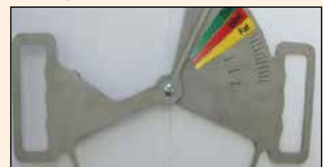
Figure 5: Sow Body Condition Caliper designed by Dr. Mark Knauer at NC State University.
