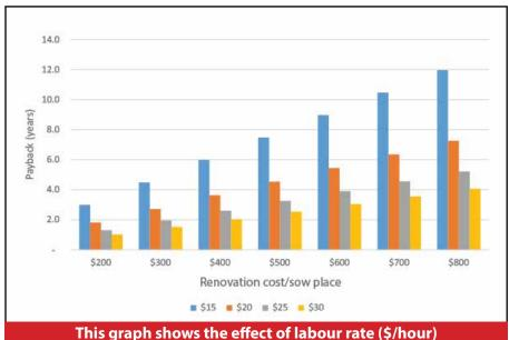
This graph shows the effect of labour rate (\$/hour) and renovation cost (\$/sow place) on payback (time) required to convert to group sow housing.
