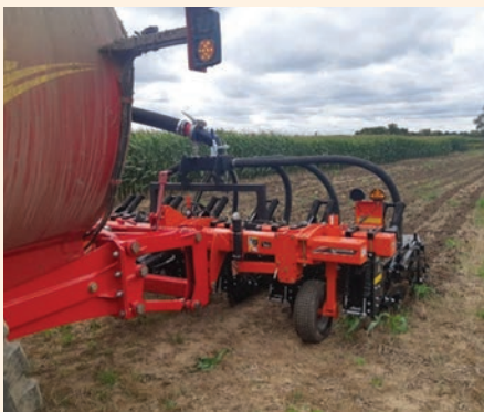
Figure 2: Manure injection with strip tiller on wheat residue
