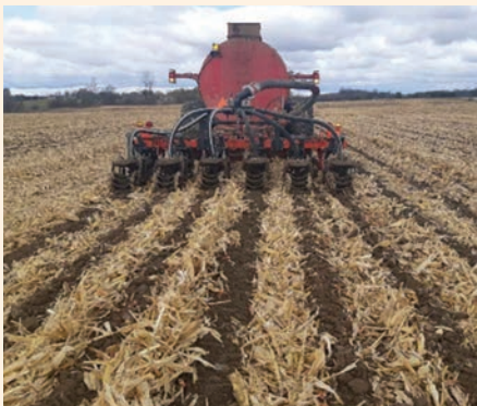
Figure 3: Fall manure injection with strip tiller after corn harvest.
