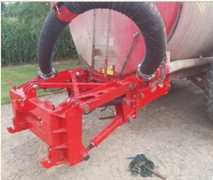
Figure 1: 3-pt quick hitch attached to manure injector lift.
