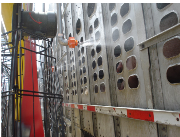
Combined water sprinkling and ventilation system.
