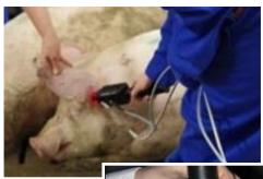
Using near infrared spectroscopy on live and carcass ears. Photos: AAFC.
