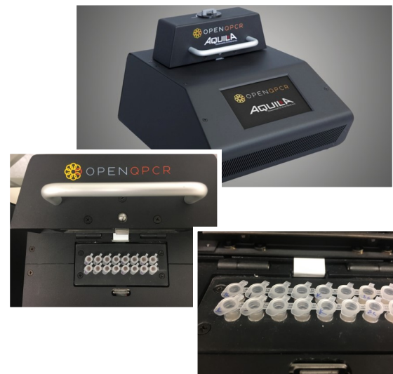
Top: The Accutas™ on-farm testing instrument is about the size of a regular household toaster. Middle: Where sample tubes are inserted. Bottom: Sample tubes. Photos: Aquila Diagnostic Systems Inc.
