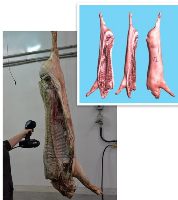
*Portable 3D scanner and carcass 3D models. Photos: AAFC*
