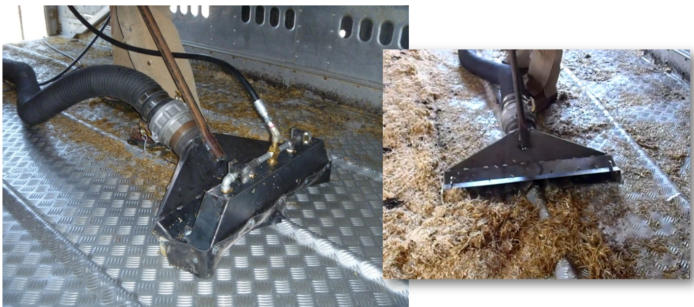
Pressure wash with vacuum ( left) compared to dry vacuum only (right) . Source: Prairie Agricultural Machinery Institute
