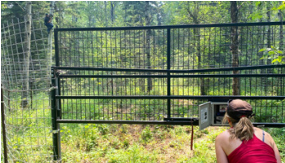
Larry climbs a tree next to the trap to ensure that the cellular signal from the mounted camera is synchronized with the trap gate mechanism below. This signal is the lifeline for the couple's phone to activate the gate, and a death sentence for the trapped sounder.
