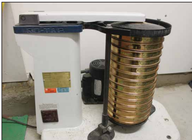
Figure 6. Rotary tap shaker with full sieve setup (left), and three-sieve hand shaking setup (right)
