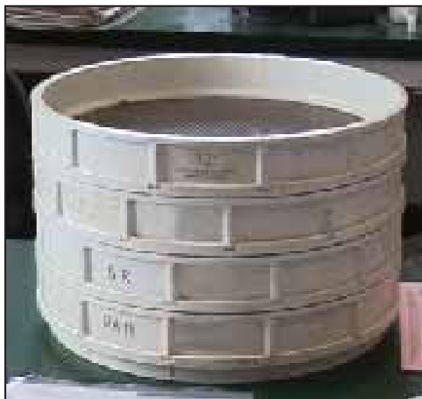
Figure 6. Rotary tap shaker with full sieve setup (left), and three-sieve hand shaking setup (right)
