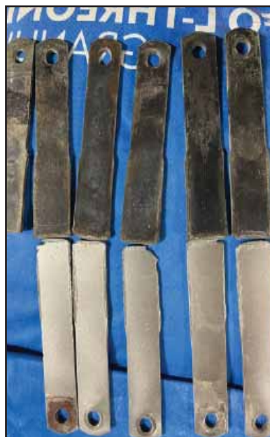
Figure 4. New hammers (top) and worn hammers (bottom) of a hammer mill (photo credit: Danilo Sotto, Western Ag Supply)
