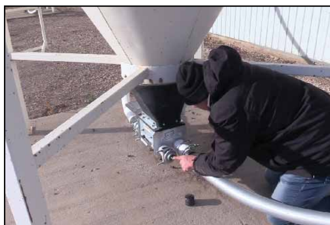
The feed bin boot and auger with motor are important components of the feed system that need regular maintenance
