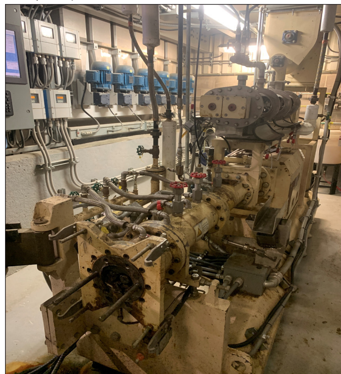
Figure 1. Extruder used for this experiment, located at the Canadian Feed Research Centre
