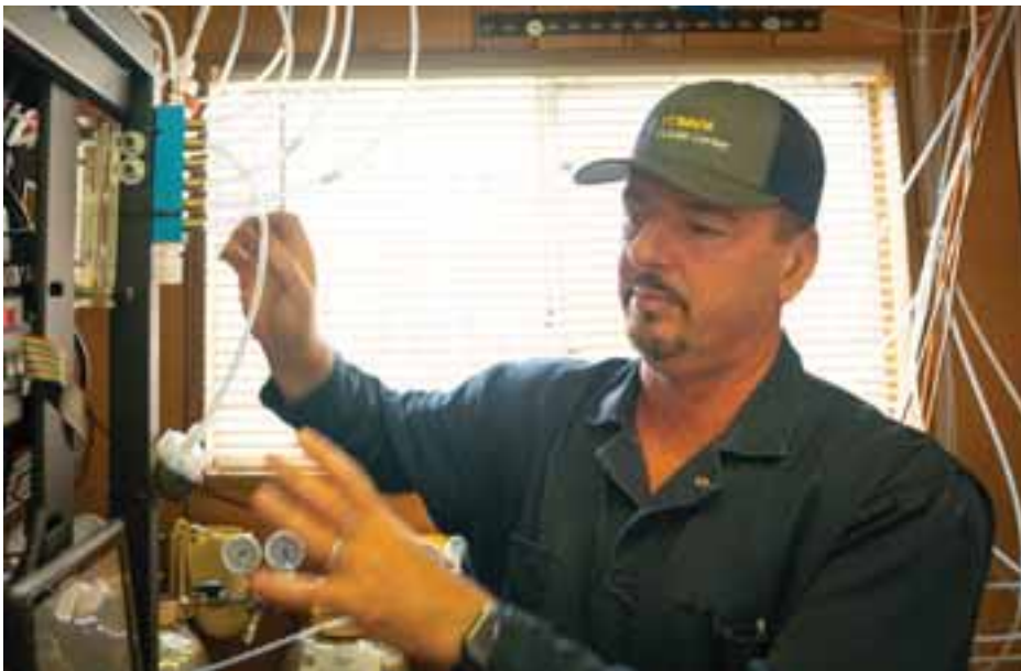
Mitloehner works with gas analyzers at the UC Davis feedlot, in preparation of a research study to measure greenhouse gases and nitrogen emissions from cattle.
