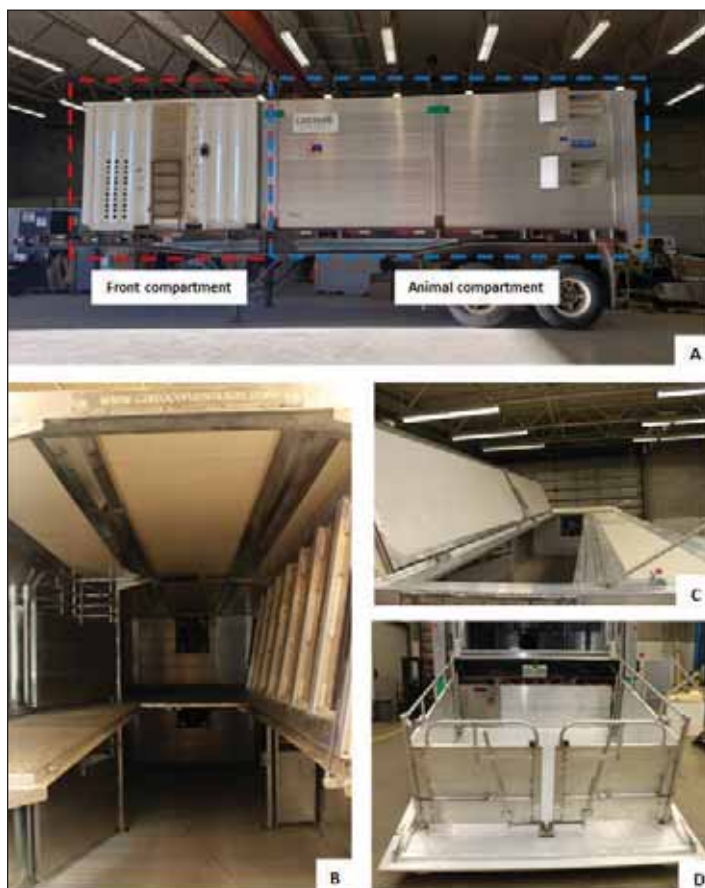
Figure 1. Photos of the prototype trailer showing the exterior of the front and animal compartment (A), its lower and upper decks (B), hinged roof (C) and hydraulic lift gate (D).
