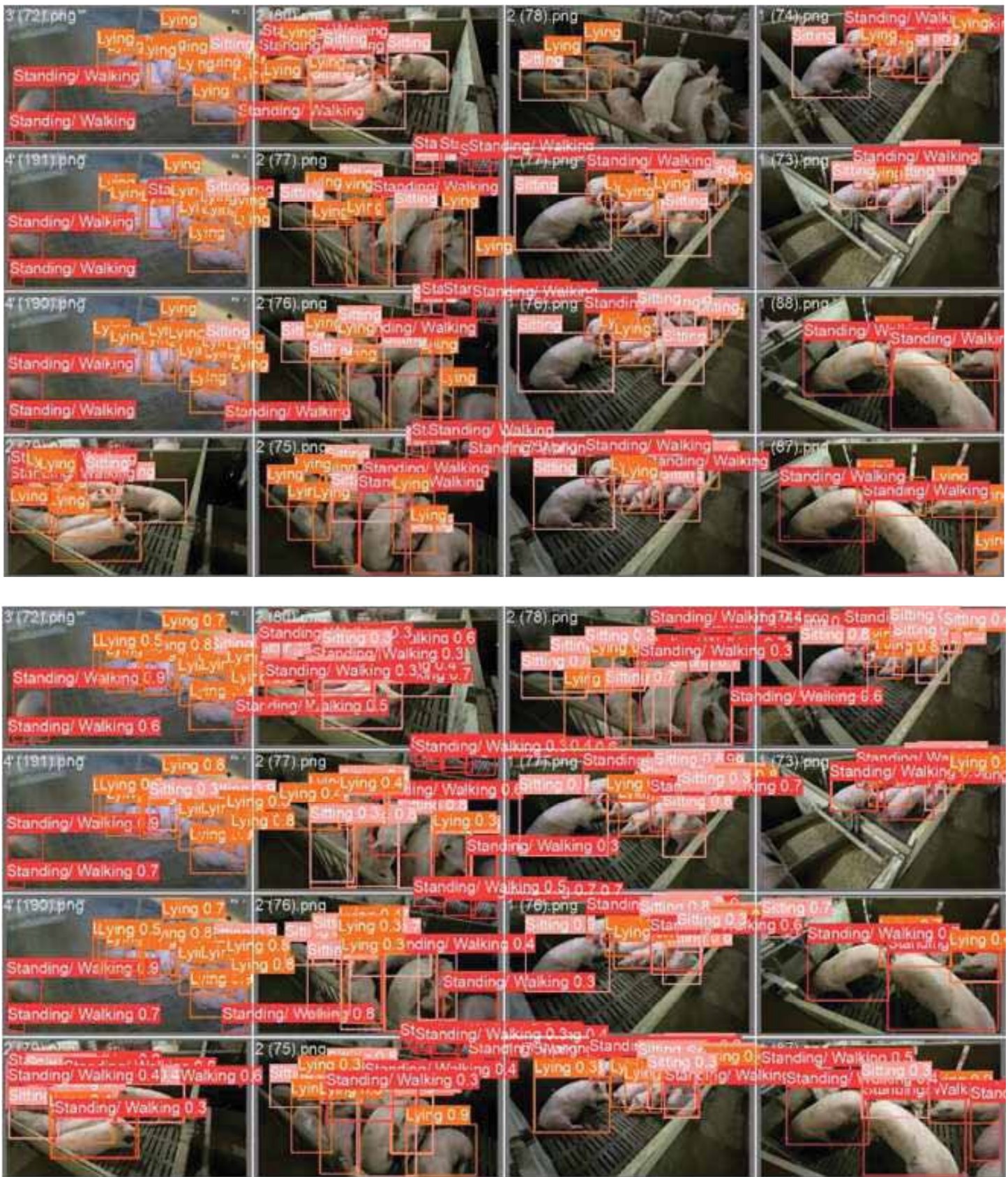
Figure 1. Qualitative analysis of YOLOv5S model showing ground truths (top) vs predictions (bottom).
